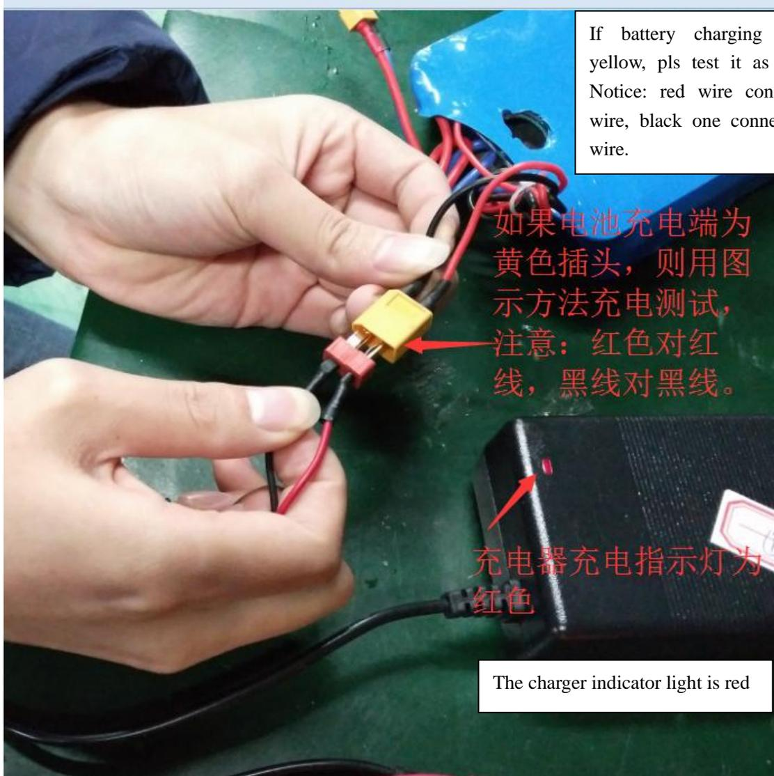
If battery charging port is yellow, pls test it as follows. Notice: red wire connect red wire, black one connect black wire.
