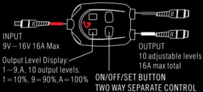
With Last-Setting memory feature. Disconnect the input plug rather then turn it off, then memory setting will start when unit is reconnected.
